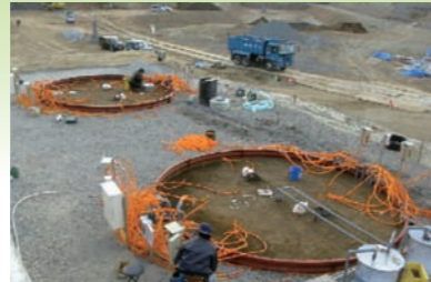
Lysimeter experiment for landfill simulation
