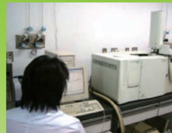
Analysis of organic contaminants using GC/MS
